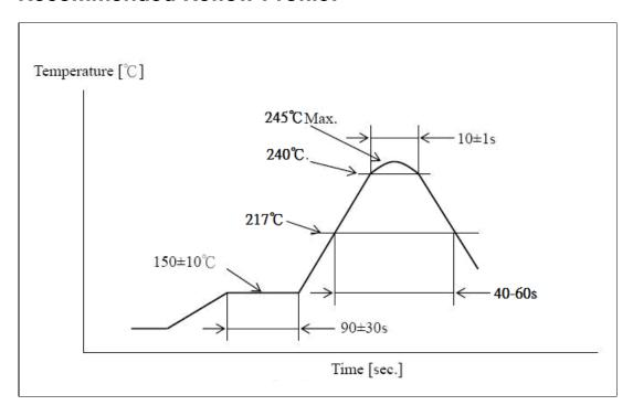
Pre heating temperature:  $150\pm10[^{\circ}C]$  Pre heating time:  $90\pm30[\sec.]$  Heating temperature:  $240\pm5[^{\circ}C]$  Heating time:  $10\pm1[\sec.]$
