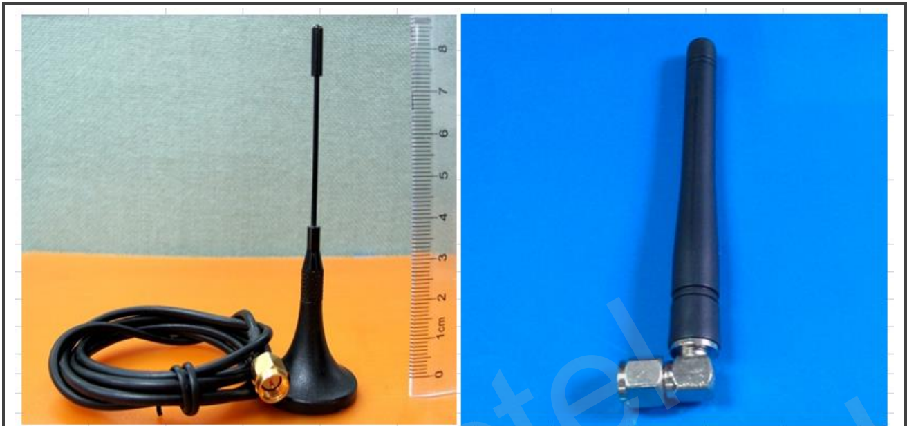
Figure 15: Example of Practical Monopole Antennas
