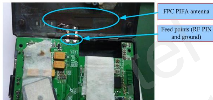
Figure 2: Example of FPC PIFA Antenna with Welding Pads and Feed Points
