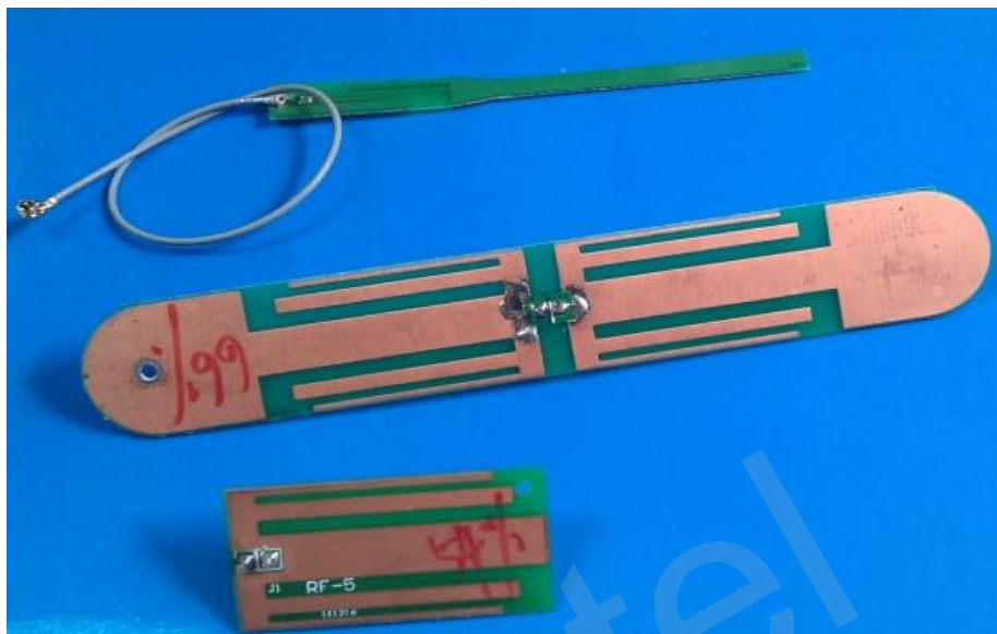
Figure 10: Example of PCB Antenna
