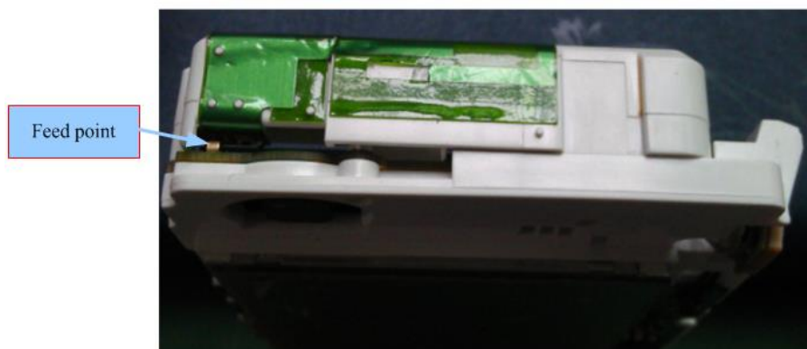
Figure 6: Example of FPC Monopole Antenna
