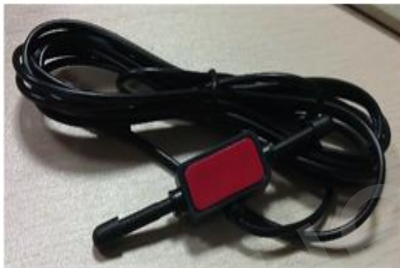
Figure 14: Example of Dipole Antenna
