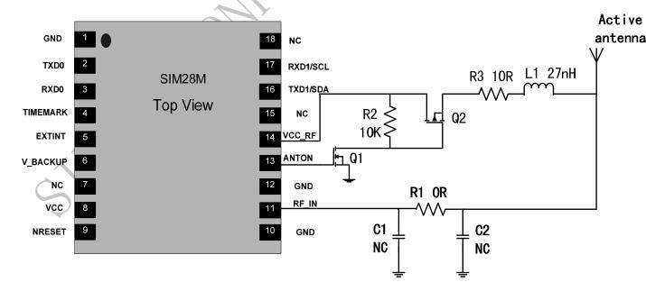
Figure 9: SIM28M Active antenna power consumption saving design
