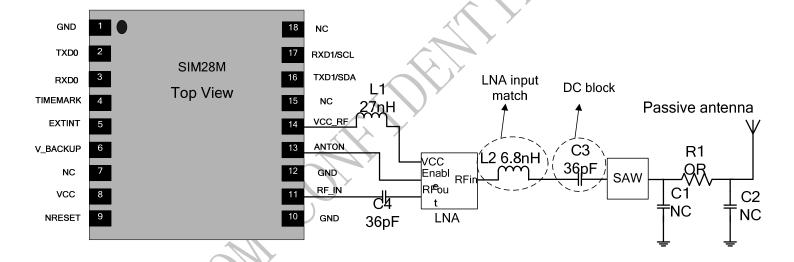
Figure 7: SIM28M passive antenna design (with external LNA and SAW)
