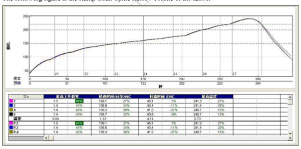
Figure 11: The Ramp-Soak-Spike reflow profile of SIM28M
