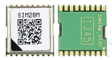
Figure 10: Top and bottom view of SIM28M
