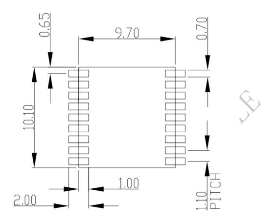
Figure 4: Recommended PCB decal (top view) (Unit: mm)
