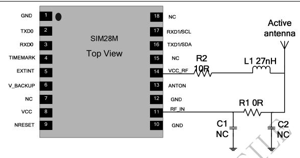
Figure 8: SIM28M Active antenna simplified design
