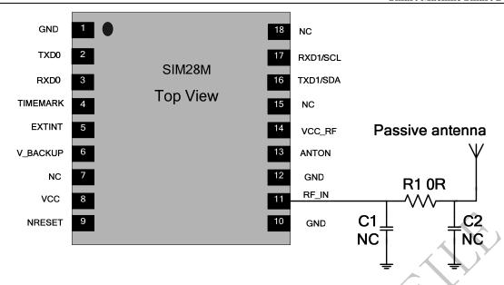
Figure 6: SIM28M passive antenna design
