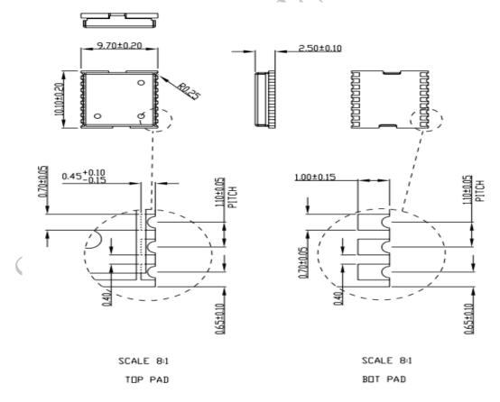
Figure 3: SIM28M mechanical dimensions (Unit: mm)
