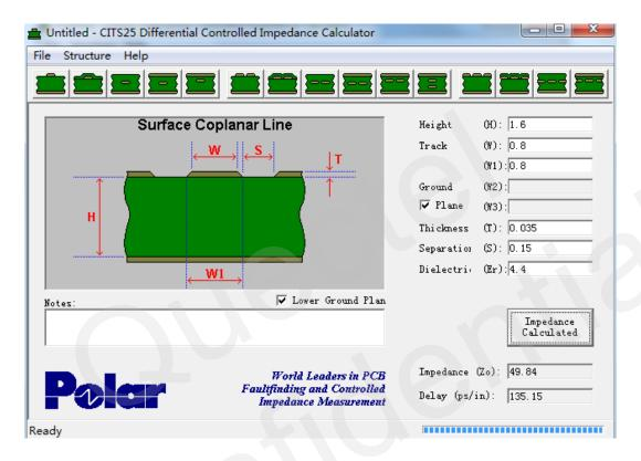
Figure 2: Structure of Coplanar WG
