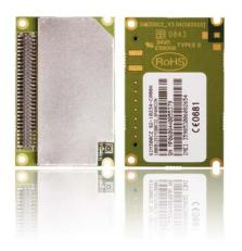
The SIM340C is a complete Quad-band GSM/GPRS solution in a compact plug-in module with DIP board-to-board connector.
