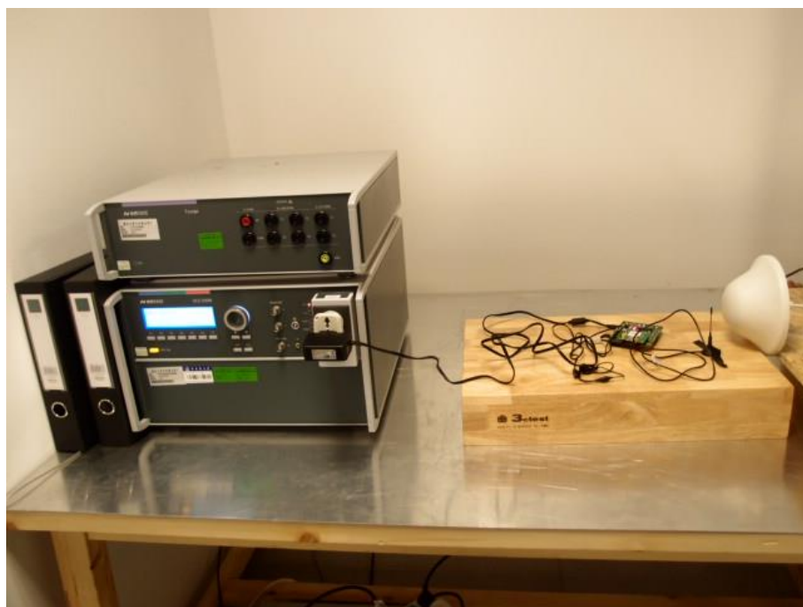
Picture 4: Photo of EFT, Surge and AC-dip test
