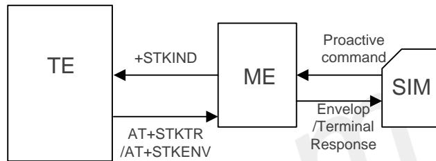
Figure 2: Basic AT command flow block diagram
