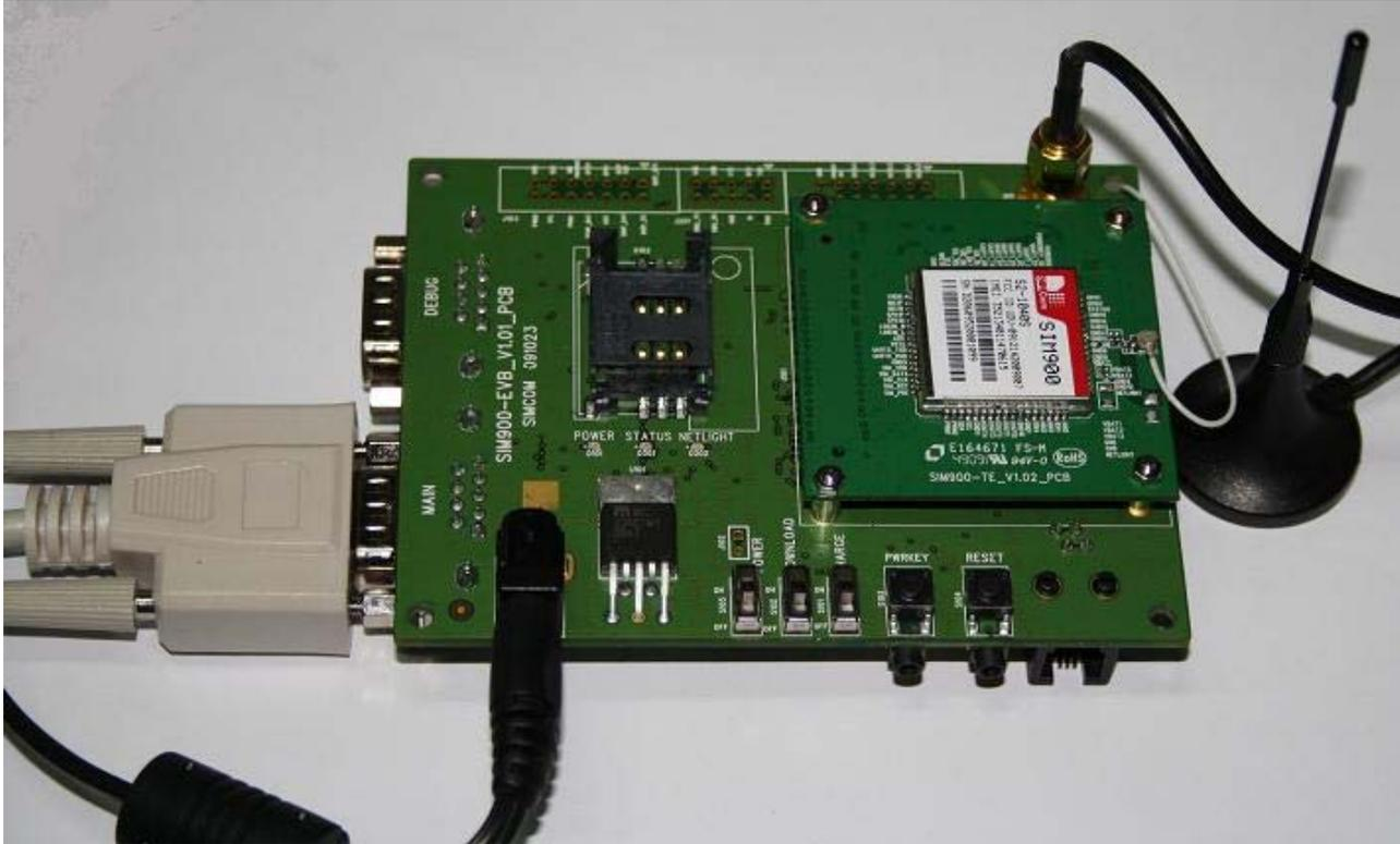
**Figure 2: Top view of SIM900 EVB**
