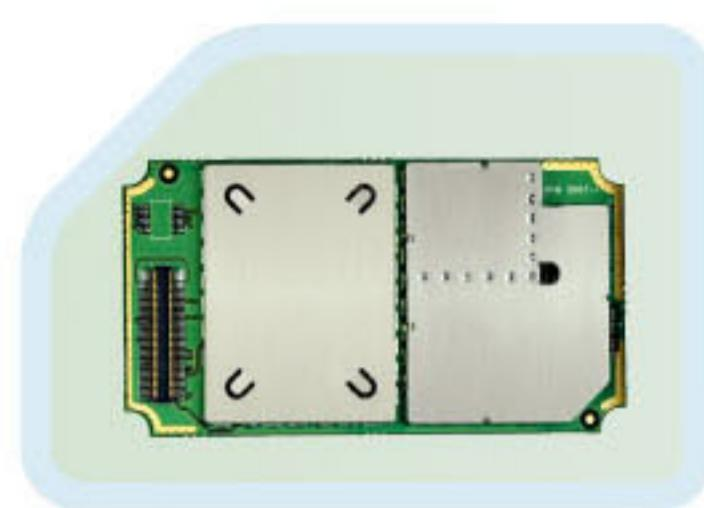
**SIM5212** is a WCDMA/HSDPA/GSM/GPRS/EDGE module solution which support up to 7.2Mbps downlink speed and 384K uplink speed data service. It also has strong capability with rich interfaces including UART, USB2.0, GPIO, I2C, TCP/IP protocol stack, etc. It is ideal for a wide arrange of products including USB modems, gateways, routers, PDAs, security solutions and much more.
