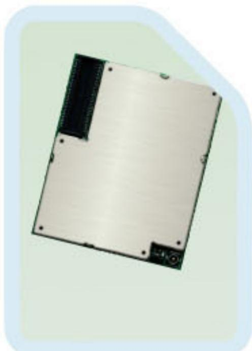
**SIM306 is a complete Tri-Band GSM/GPRS solution in a compact plug-in module. The leading features of SIM306 make it ideal for virtually unlimited application, such as WLL applications, M2M applications, handheld devices and much more.**
