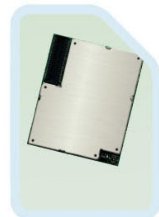
The SIM300/340 is a Tri-Band/Quad-Band GSM/GPRS solution in a compact plug-in module.
