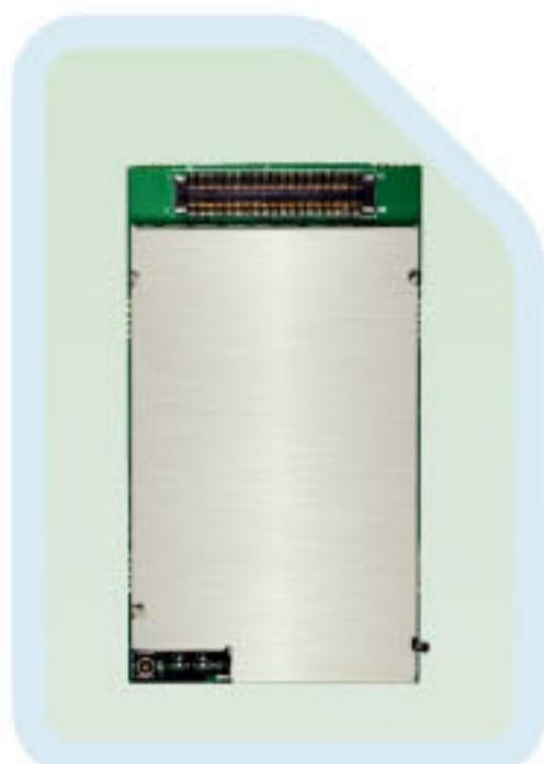
**SIM4100** is a dual-mode TD-SCDMA module which works at 2010-2025MHz on the TD-SCDMA mode and Tri-Band 900/1800/1900MHz on the GSM mode. The leading features of **SIM4100** make it ideal for virtually unlimited applications, such as WLL applications (Fixed cellular terminal), M2M applications, handheld devices, PC card and much more.
