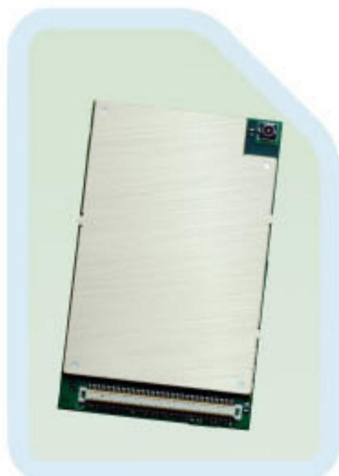
**SIM600** is a complete Quad-Band GSM/GPRS/EDGE solution in a compact plug-in module which is ideal for virtually unlimited applications, such as WLL applications (Fixed Cellular Terminal), M2M applications, PC card, USB modem, and much more.
