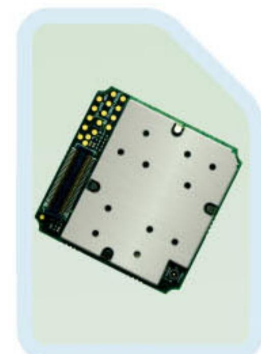
**SIM5210** is a HSDPA/WCDMA/GSM/GPRS/EDGE module solution which support up to 7.2M downlink speed and 384K uplink speed data service. It also has strong capability with rich interfaces including UART, USB2.0, GPIO, I2C, TCP/IP protocol stack, etc. It is ideal for a wide arrange of products including USB modems, gateways, routers, PDA, security solutions and much more.
