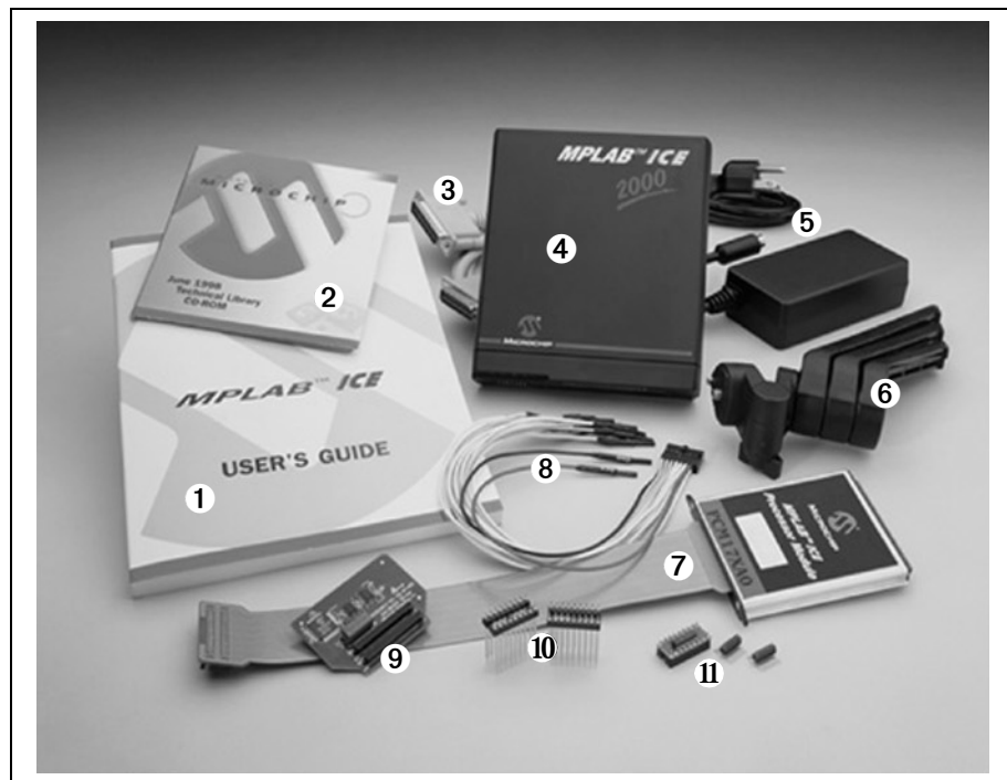
Figure 1.2: MPLAB ICE Emulator Kit and Optional Hardware
