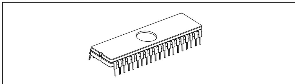
2. Place the device in an Ultraviolet (UV) EPROM Eraser. The amount of time required to completely erase a UV erasable device depends on: the wavelength of the light, its intensity, distance from UV source and the process technology of the device (the size of the memory cells).
