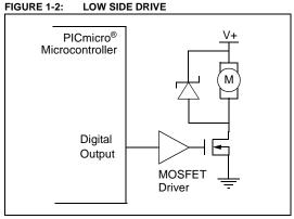
This is the lowest cost drive technique because of the MOSFET drive simplicity. Most applications can simply use an output pin from the PICmicro microcontroller to turn the MOSFET on.
