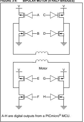
FIGURE 3-4: **BIPOLAR MOTOR (4 HALF-BRIDGES)**
