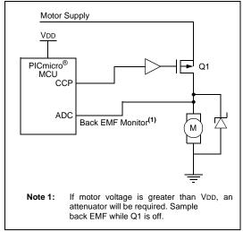
FIGURE 7-1: BACK EMF MOTOR SPEED SENSING
