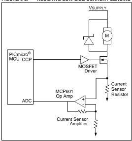
FIGURE 6-2: RESISTIVE LOW SIDE CURRENT SENSING
