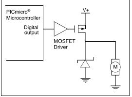
This drive can control a Brushed DC motor in one direction. This drive is often used in safety critical applications because a short circuit cannot turn the motor on.
