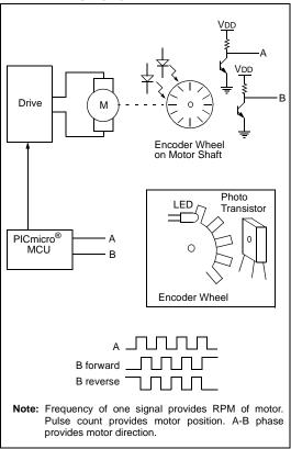
Quadrature sensing can easily be accomplished in software, but there is generally an upper limit to the RPM. By using a few gates, the sensing can be done partially in hardware and partially in software. The new PIC18FXX31 and dsPIC<sup>®</sup> 16-bit Digital Signal Controller families include an encoder interface that allows MUCH higher RPM motors to be measured with an excellent degree of accuracy.
