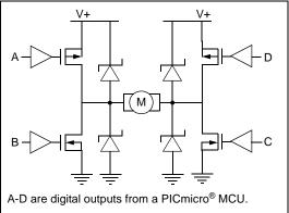
The H-bridge derived its name from the common way the circuit is drawn. This is the only solid state way to operate a motor in both directions.
