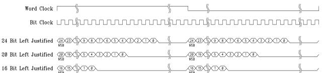
The data is read into the 24 LSBs of the 28-bit internal datapath and sign-extended into the upper bits to create a 28-bit number, resulting in the ADC having an effective range of +0.5 to -0.5.
