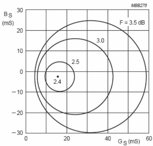
$I_C = 14 \text{ mA}; V_{CE} = 10 \text{ V}; f = 800 \text{ MHz}.$
