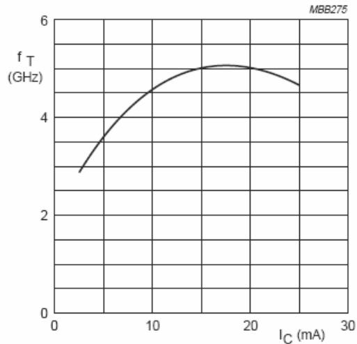
$V_{CE} = 10$  V;  $f = 500$  MHz;  $T_{amb} = 25$  °C.
