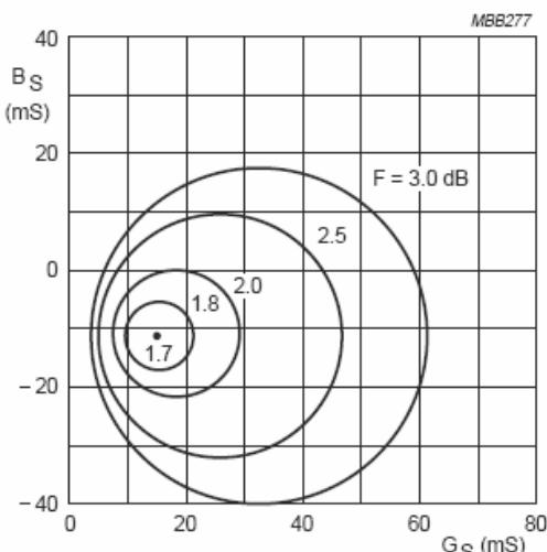
$I_C = 4 \text{ mA}; V_{CE} = 10 \text{ V}; f = 800 \text{ MHz}.$
