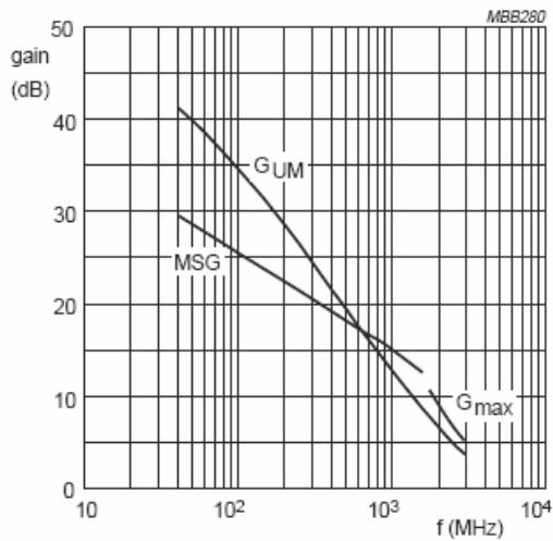
$I_C = 5 \text{ mA}; V_{CE} = 10 \text{ V}.$
