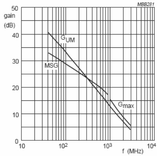
$I_C = 15 \text{ mA}; V_{CE} = 10 \text{ V}.$
