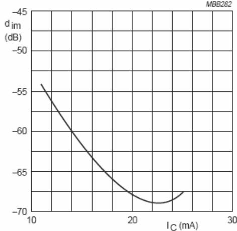
$V_{CE} = 10 \text{ V}$ ;  $V_O = 150 \text{ mV}$  (43.5 dBmV);
